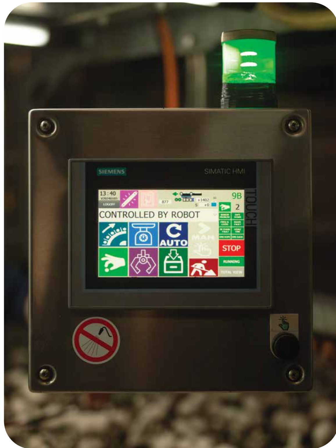
ABOVE: The installation of Mycronics MDH20, serial number 00001, represented a decade of engineering challenges. The system needed to be finely calibrated yet low maintenance and easy to operate—even the screen icons were custom designed. It also had to be food-safe (meaning no lubricants) and resilient to human error, while withstanding a tough environment that includes steam cleaning, i.e. robot kryptonite.
