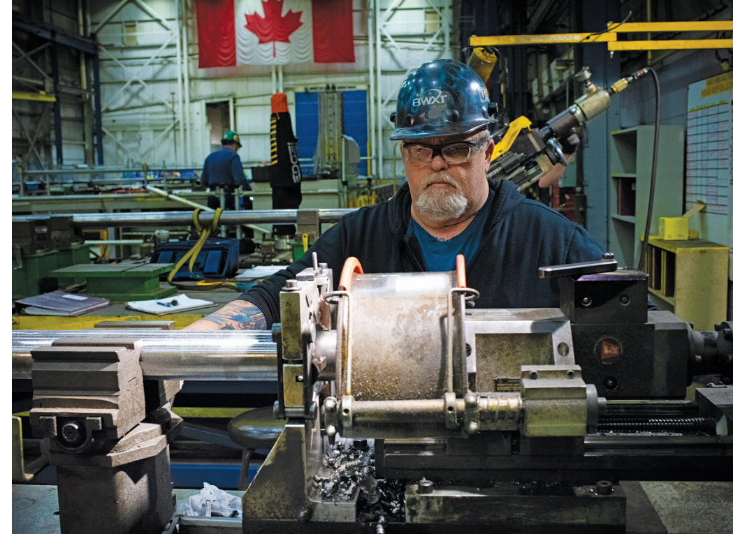
Feeder machining in the nuclear industry involves specialized techniques and equipment to fabricate and maintain the feeder pipes that carry coolant within nuclear reactors.
