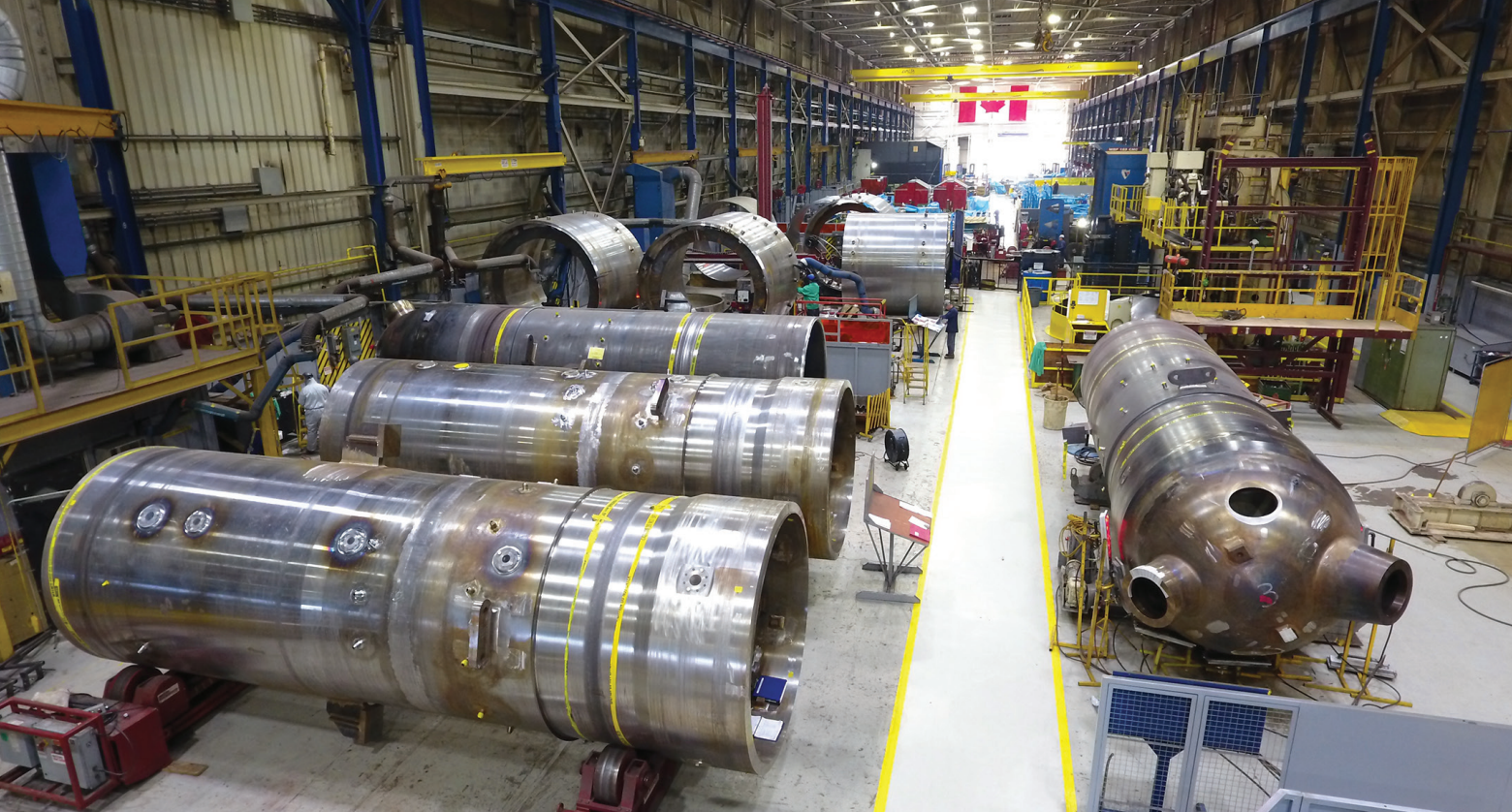
BWXT has been involved in CANDU reactor refurbishments, such as the manufacture of steam generators, for Bruce Power.
